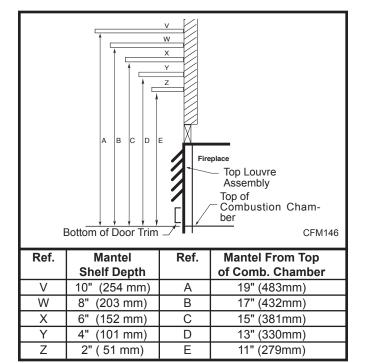
Fig. 3a Combustible mantel minimum installation.
